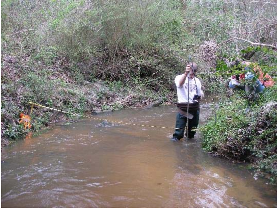
40 Figure 20 Price AA Current Meter being used in the field
