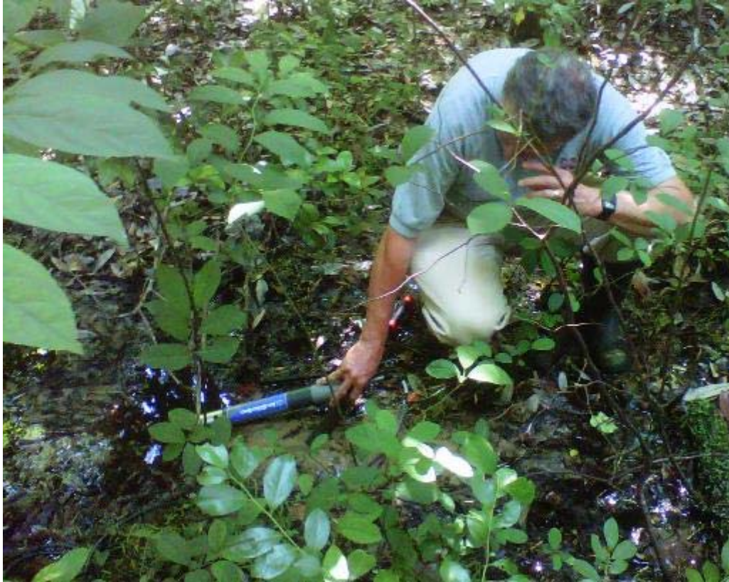
Figure 27 In-Situ, Inc. Troll 9500 multi-parameter sonde being used to measure field water quality parameters of a spring
