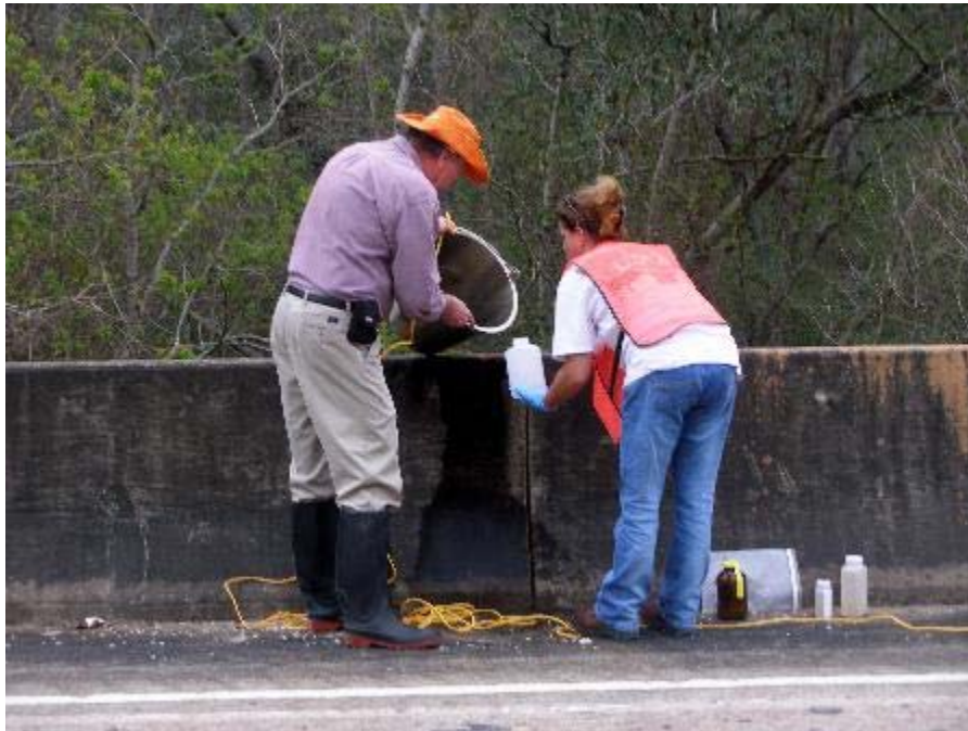
Figure 23 Stream water samples being taken from bridge-side using a stainless steel pale
