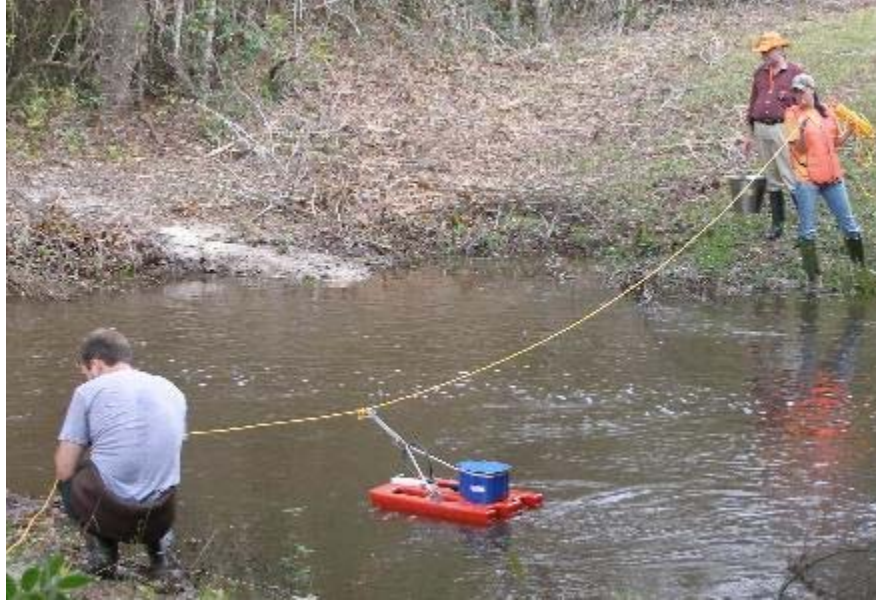
Figure 11 StreamPro RDI Doppler Unit at use in the field
