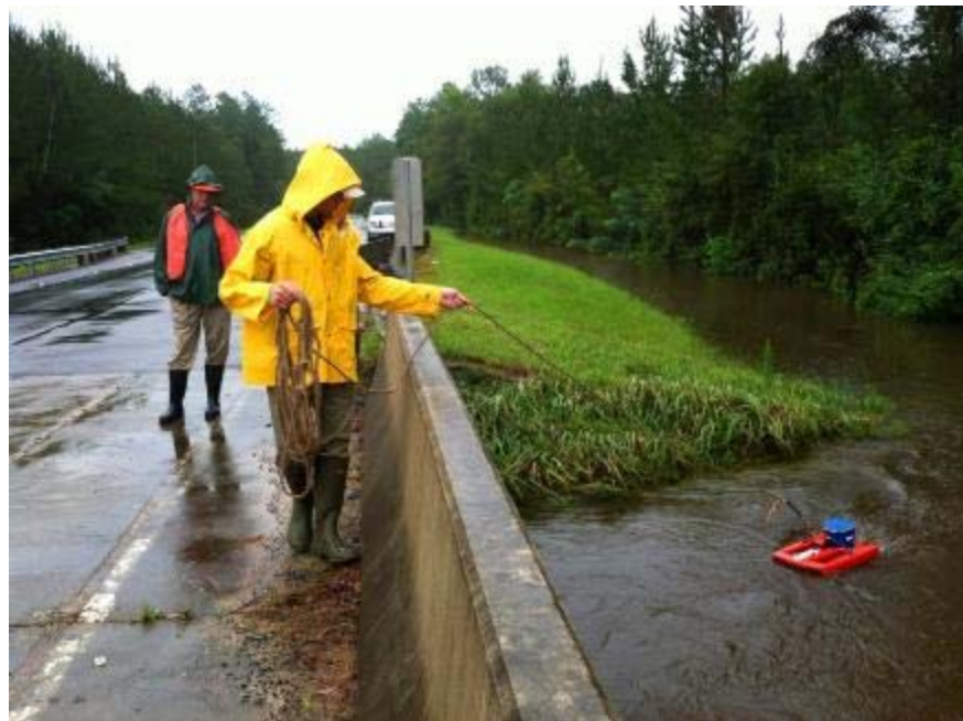
Figure 12 StreamPro RDI Doppler Unit at use in the field
