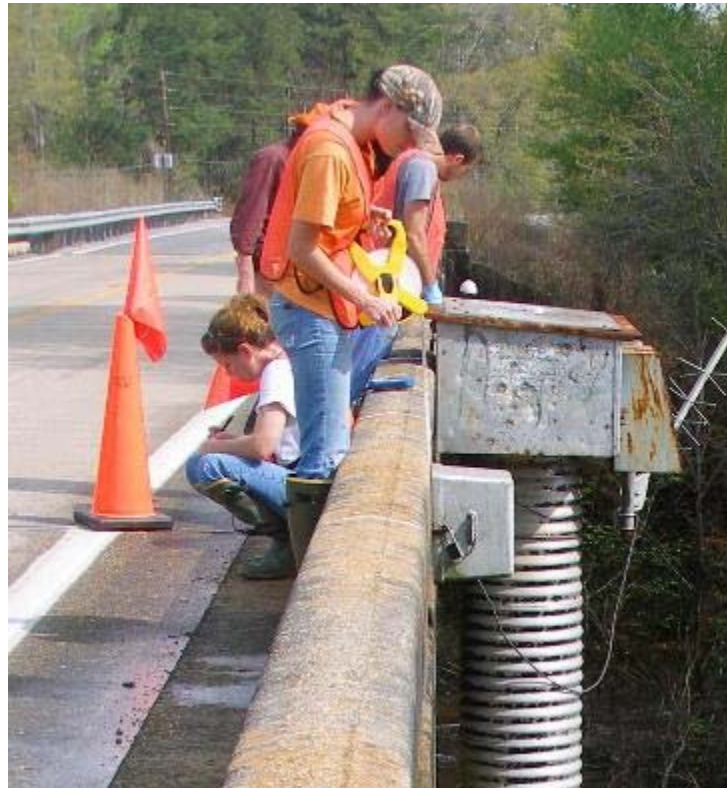
Figure 10 Measuring tape being used to measure stream stage from bridge railing
